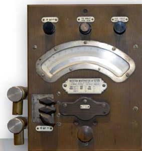
| Watt-meter manufactured by General-Vertreter Wien, from 1907
