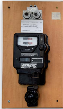
Coin-operated meter Landis & Gyr from 1938
